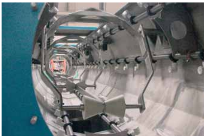
Pipe support with central height adjustment
